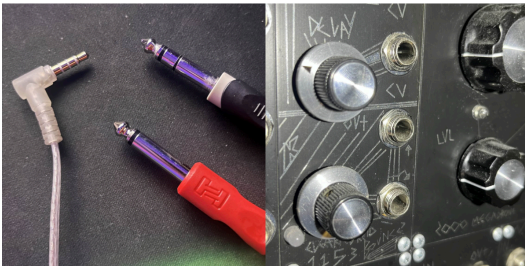
Figure 3.6 Male & Female 1/4" Audio Connectors (male 3.5mm for reference). Image Source: Author
